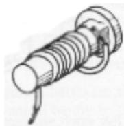
Figure 4: Using an electromagnetic with a core of ferromagnetic material.
